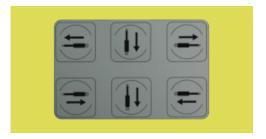
If the distribution device is equipped with the hydraulic movement of the arms, these related movement keys are enabled for movement management of the three-way electro-hydraulic control unit.
