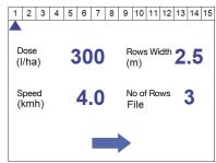
The **EPA 2.0** system calculates the best hole in the yellow flow rate calibration disc to obtain the correct delivery.
